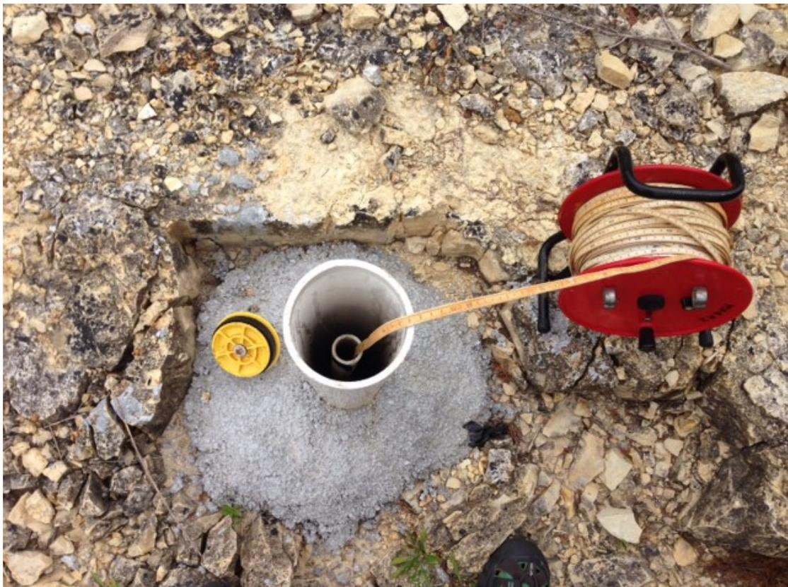
Figure 7: Making water level measurements.
